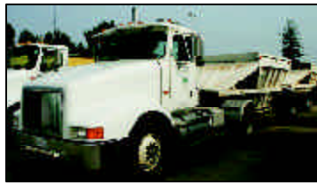
Asphalt hauling and spreading truck
